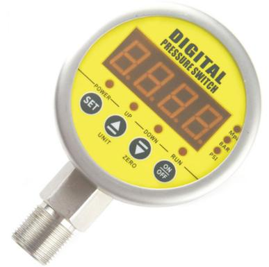
MD-S828EA is a intelligent digital pressure switch, setting pressure measurement, pressure display, control in one professional unit. It can be set two groups relay signal. About output signal, 4-20mA and Rs485 are available.
